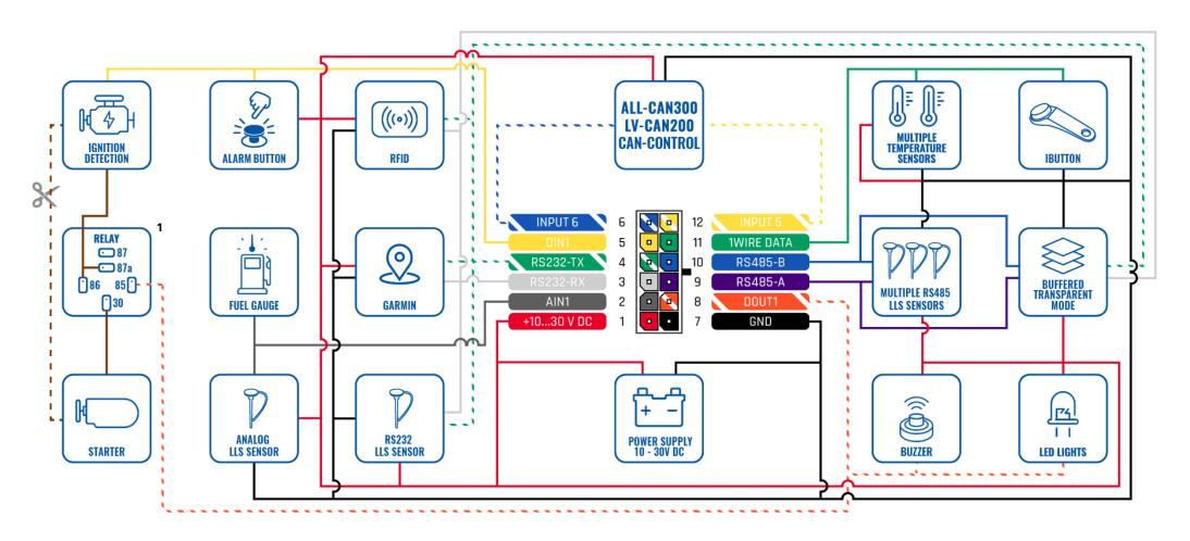
Figure 3 FMB125 Wiring scheme
