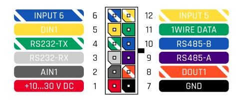
Figure 2 FMB125 2x6 socket pinout
