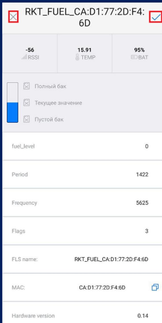
Figure 16 - Saving BLE FLS changes and disconnecting from the sensor.
