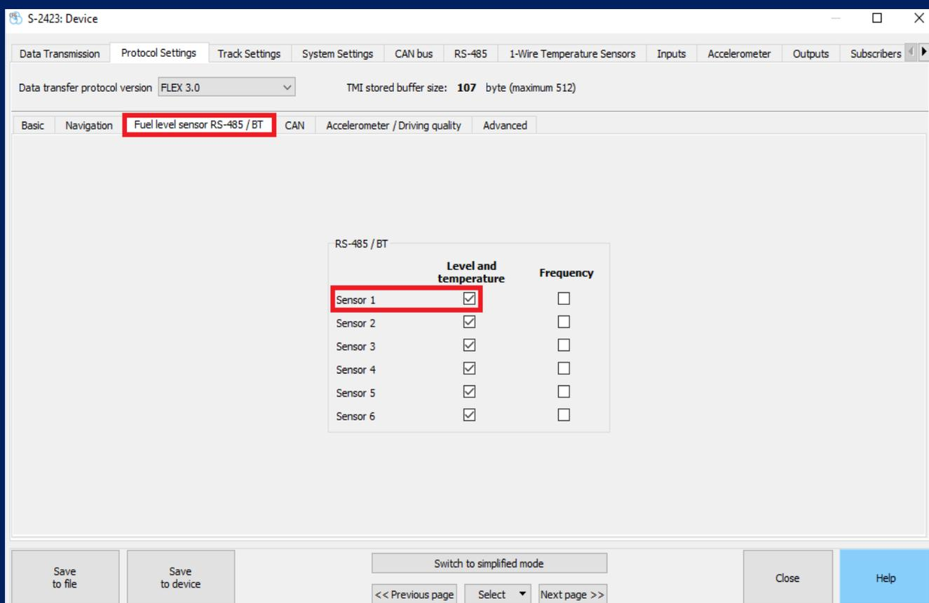
Figure 26 - Configuring the display of BLE FLS parameters
