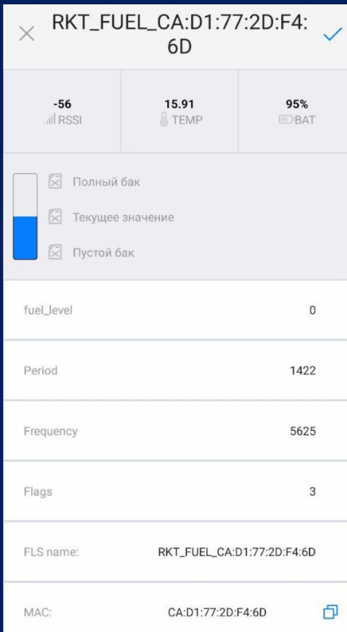
Figure 9 - BLE FLS setup window
